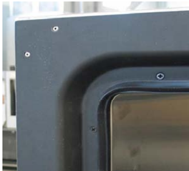
Chamber side thermal break
